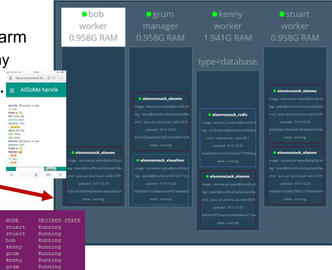
The screenshot shows a Docker Swarm interface with four nodes: bob (worker), grum (manager), kenny (worker), and stuart (worker). Each node has a service named 'alsomestack\_alsome' running. A red arrow points from the 'alsomestack\_alsome' service on the 'stuart' node to a terminal window at the bottom left displaying the command 'root@grum:~/proj# docker stack ps alsomestack' and its output.
